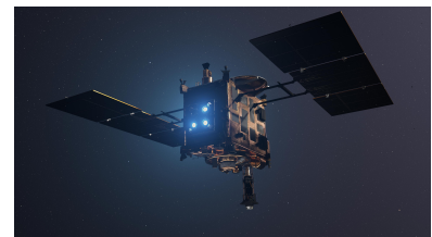
Figure 2: The Hayabusa 2 spacecraft with three ion engines operating.
