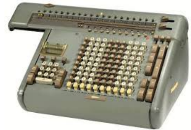
Figure 5: The human computers at NACA, later NASA, used Friden calculators. These bulky machines could do basic arithmetic, which was cutting edge at the time.
