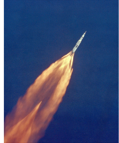
Figure 1: The exhaust plume of the Saturn V launch vehicle. The exhaust is under-expanded , which is why the plume extends far beyond the exit area of the rocket nozzle. We'll learn about why this happens later in the lecture!
