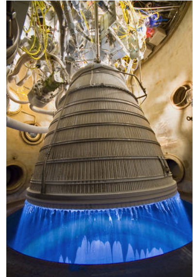
Figure 1: Operational liquid bi-propellant rocket engine on a test stand. The converging-diverging nozzle accelerates the hot combustion gases to supersonic speeds. We'll learn about why rocket nozzles are shaped this way later in the lecture!
