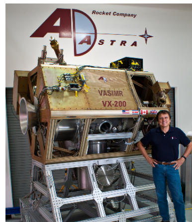
Figure 10: A prototype of the Variable Specific Impulse Magnetoplasmadynamic Rocket (VASIMR).
