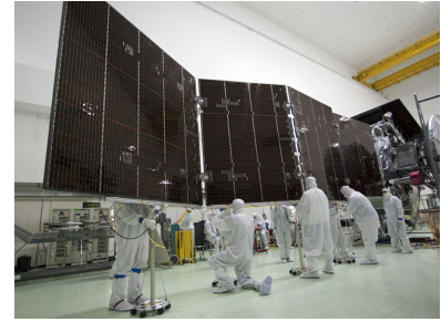
Figure 4: Solar panels under preparation for the Juno spacecraft.
